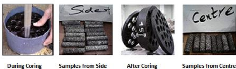
Figure 4.4 Torsional Bars Extraction SGC Fine Aggregate Matrix
