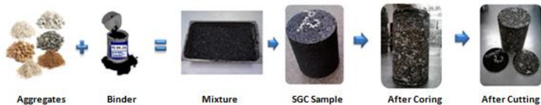
Figure 3.1 Sample Fabrication of Asphalt Concrete Mixtures
