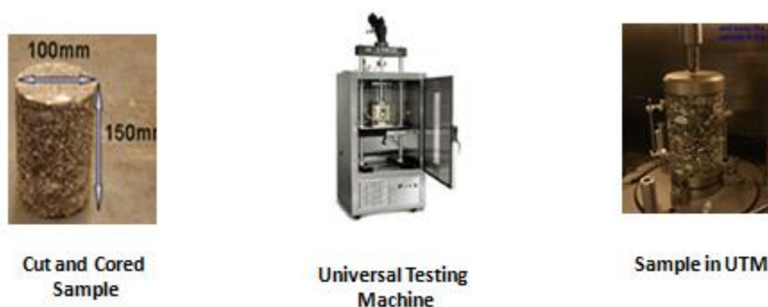
Figure 3.3 Installing the Asphalt Concrete Samples for Tests
